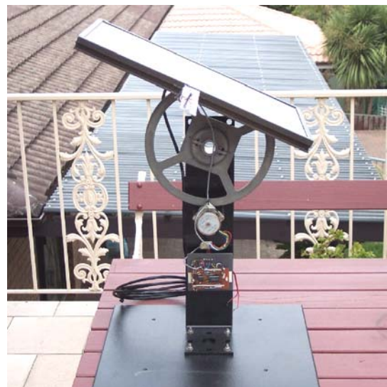
Fig. 5 A prototype solar tracker
